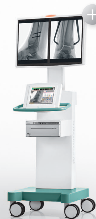
Option 3: Ziehm Viewing Station The C-arm can be easily supplemented with an extra Viewing Station featuring a 24" landscape splitscreen monitor or dual 19" flatscreen monitors.
